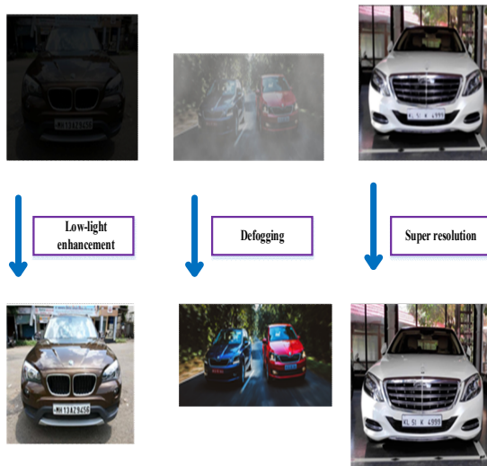
Figure 6. Three Different Image Preprocessing Techniques' Visual Effects Include Low-Light Enhancement, Defogging, And Super-Resolution.
