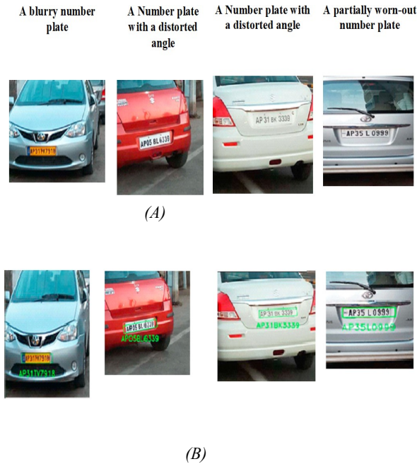
A) Images Of A Test Case For The Angled And Distorted Number Plate. B) The Results Of Detection And Recognition Of The Number Plate Across All Test Cases.
