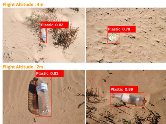
Fig. 8. Examples of Plastic Litter Detection Using YOLOv8
