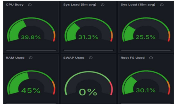
Fig. 6.6 Sequential Execution System Metrics (8gb System)
