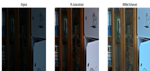
Fig.6. Image Preprocessing of Original to PIL Autocontrast to MIRNet enhanced Images
