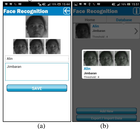
Figure 7: Enrollment Display : (A) Training Face Input (B) Threshold Calculation
