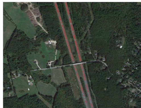
Fig.4. Proposed Road Extraction Result For Satellite Image 1
