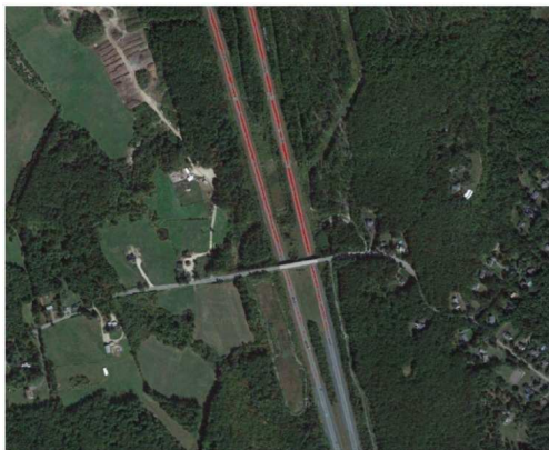
Fig. 5. Existing Road Extraction Result For Satellite Image 1
