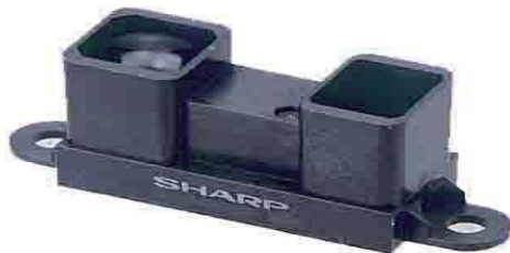
Figure 5: GP2Y0A02YK0F Infrared Sensor
