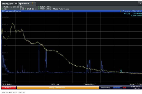
Figure 30: The Spectrum Of Masking Noise Created By The Noise Generator "LGSh-503"
