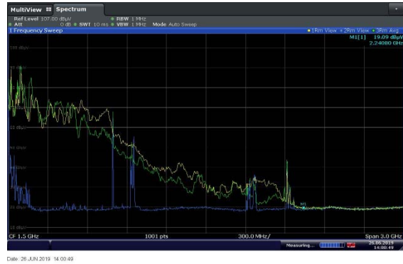
Figure 32: The Spectrum Of Masking Noise Created By The Noise Generator "Gnome-3"
