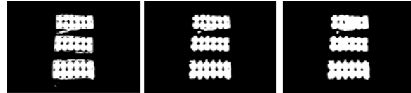
Figure 16: The Process Of Improving Images With Morphological Transformation
