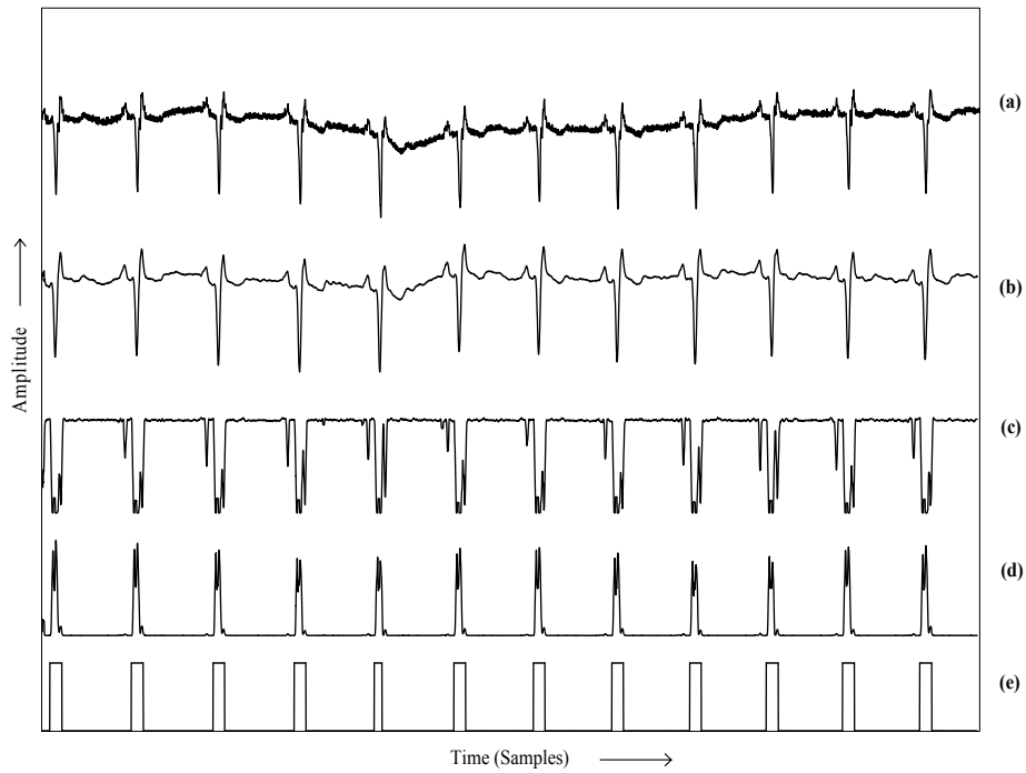
Fig.3 QRS detection of record MO1_036 of CSE database, (a) Raw ECG, (b) Filtered ECG, (c) Entropy QRS, (d) Entropy non-QRS, (e) QRS Detection by SVM
